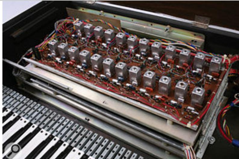
With only two master oscillators, the String Symphonizer was a cut-down design compared with Ken Freeman's Prototypes #2 and #4.
