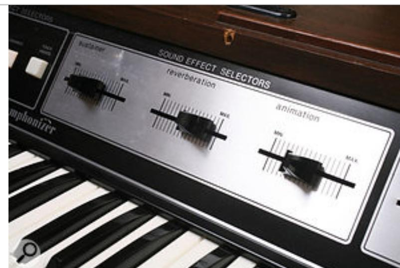
One of the most important String Symphonizer parameters was Animation, which introduced vibrato to the first oscillator band. The instrument also featured an internal spring reverb.
