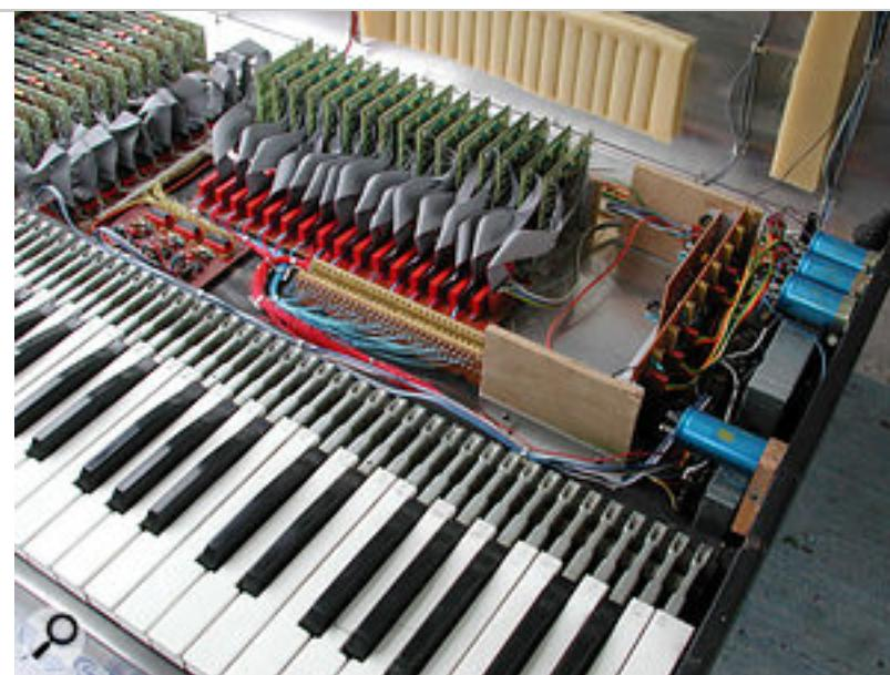
Prototype #4 was fully polyphonic, with three master oscillators and some sophisticated innovations including the use of digital delay lines for vibrato.
